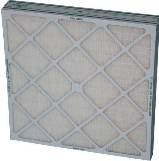
The Camfil Farr Opti-Pac provides high efficiency air filtration in a space saving 4" deep filter pack that can reduce valuable in-line air handler component depth and reduce inventory space requirements. Light weight and easy to handle, the Opti-Pac is available in efficiencies of MERV 11, MERV 13 and MERV 14 per ASHRAE Standard 52.2.
